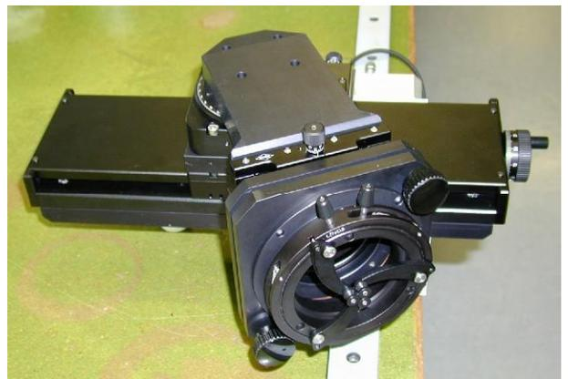
The pictures above show an example of a special holder which could be easily adapted for these rotation measurements by inserting an additional rotation table behind the 3-finger-clamp.
